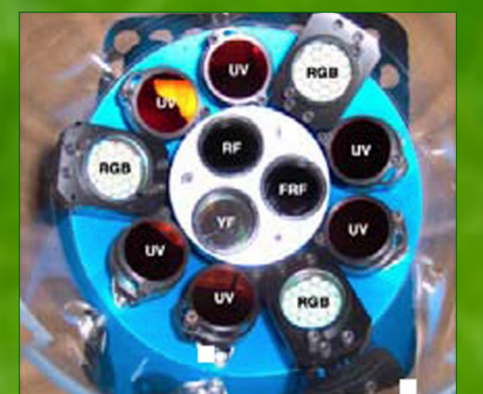
Fig.2 Led (UV = ultravioletto; RGB = red-green-blu) e fotodiodi rivelatori (YF = yellow fluorescence; FRF = far red fluorescence; RF = red fluorescence) costituenti il Multiplex®.
